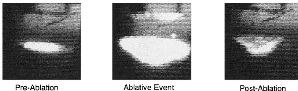
Fig. 3. The left (control) image shows the surface of the gelatin by using a low energy (subablative) pulse. The middle image was taken during the ablation attempt. The right image, measured with a low-energy pulse, shows crater formation on the surface of the gel. Pulse energies below threshold showed no changes in the surface.
