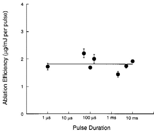
Fig. 5. The ablation efficiencies of the 1-μsec, 50-μsec, 100-μsec, 150-μsec, 2-msec, 5-msec, and 10-msec pulses. All fibers used were 300 μm. All experiments were conducted at 1 Hz. The ablation efficiencies agree ( $P < 0.05$ ).
