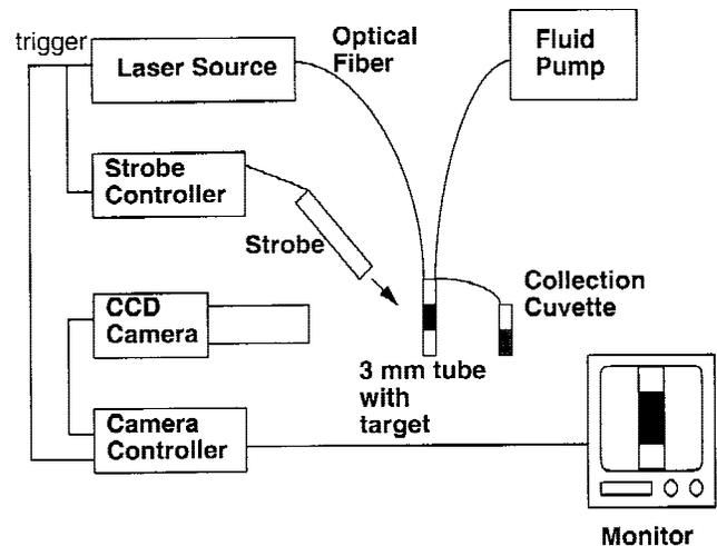
Fig. 2. Experimental setup for ablation threshold detection and ablation efficiency experiments. The laser sources were the 1- $\mu$ sec, 100  $\mu$ sec, and the millisecond lasers. The CCD camera was used to monitor fluorescence for detection of ablation threshold. The fluid pump flushed the target of ablated material, which was collected into the cuvette. The cuvette contents were later analyzed for ablation mass.
