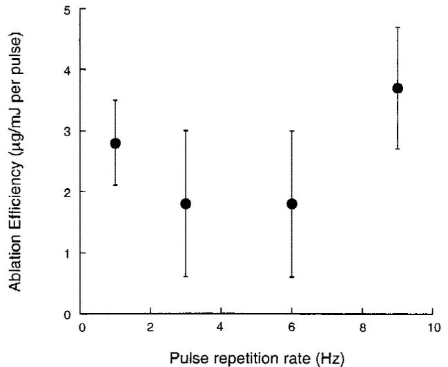
Fig. 7. The effect of pulse repetition rate on clot ablation efficiency. The fiber size was 300 μm. The pulse duration was 100 μsec. All ablation efficiencies agree ( $P < 0.05$ ).
