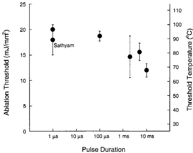
Fig. 4. Ablation thresholds for 1 μsec, 100 μsec, 2 msec, 5 msec, and 10 msec. All fiber sizes were 300 μm except for the 1-μsec pulse, which used a 100-μm fiber. The ablation thresholds all agree ( $P < 0.05$ ).
