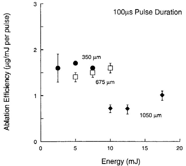
Fig. 6. The dependence of spot size on ablation efficiency. A 100-μsec pulse was used. The ablation efficiency of the 350-μm and 650-μm spot sizes agree ( $P < 0.05$ ). The ablation efficiency of the 1,050-μm spot is lower than that of the smaller spots ( $P < 0.05$ ).
