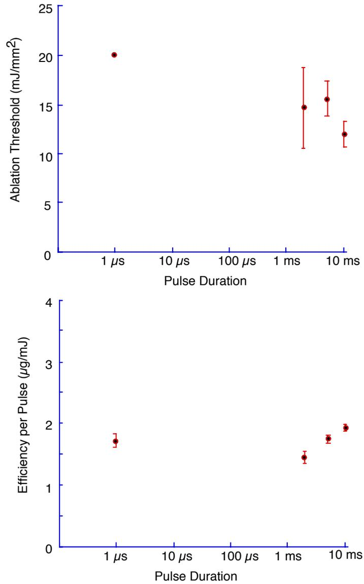
**Figure 2.** (Top) The ablation thresholds for microsecond and the millisecond pulses. (Bottom) The ablation efficiencies for the microsecond pulse and the millisecond pulses. The average and standard deviations of five samples at each millisecond pulse duration are shown.
