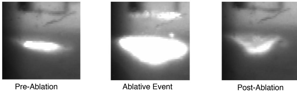
**Figure 1.** The subthreshold pulse has fluorescence indicating the undisturbed gel surface (left). The ablative pulse (middle). A subsequent subthreshold pulse indicates a lower surface due to ablation (right).
