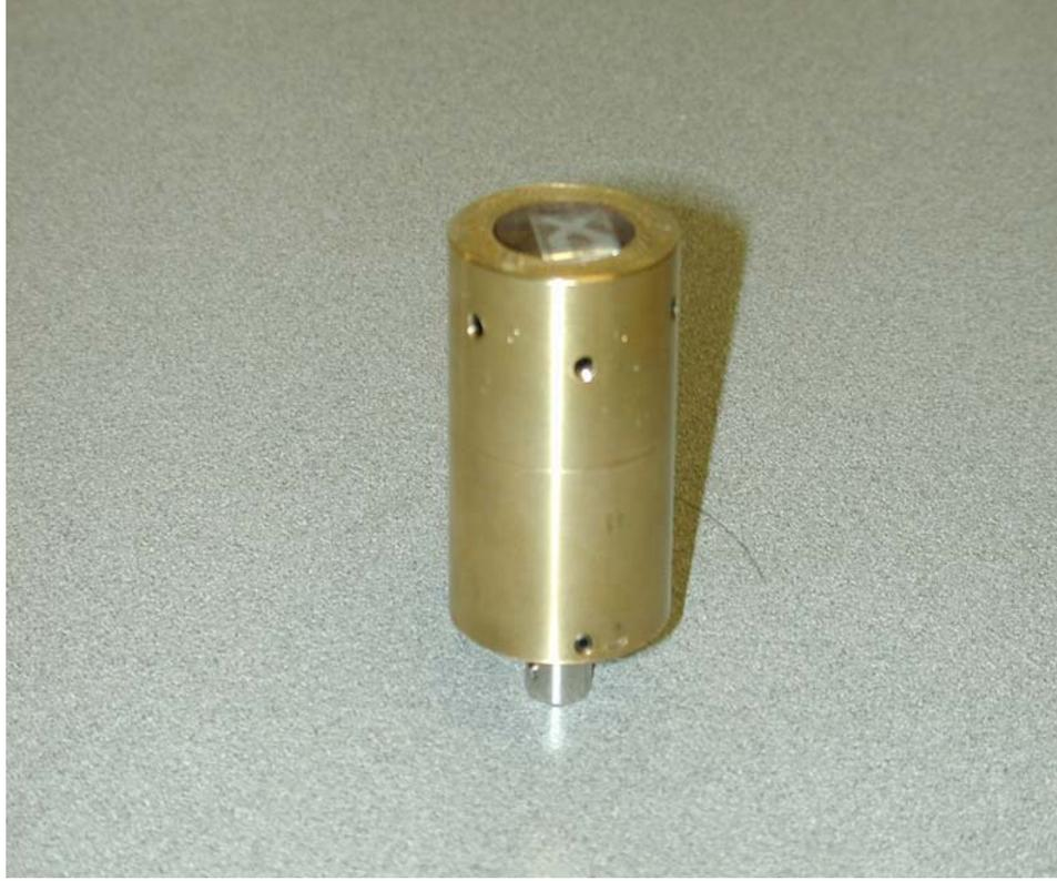
**Figure 3.** The acoustic transducer was a PVDF film detector in a brass housing. A BNC was connected to the PVDF electrodes for coupling to the oscilloscope. The active area is shown as the crossed region on the top of the transducer.
