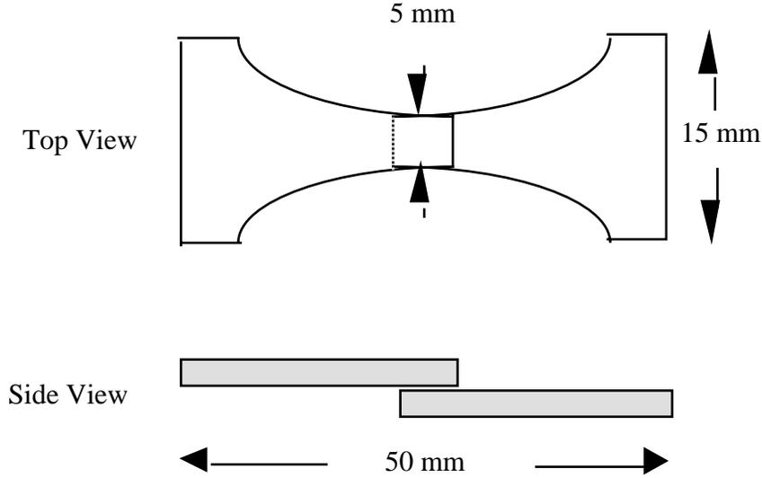
**Figure 1.** Dog bone shaped die mold used to section the aorta and intestine samples for mechanical testing.
