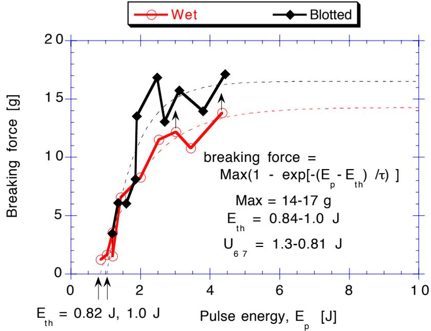
Figure 5: Weld strength vs laser pulse energy. The weld strength is expressed as the load (g) at which the weld broke. The wet and blotted tissues were not significantly different in their behavior. (The two arrows indicate two welds where the heterograph broke before the weld broke, and hence these data are lower-limit values for the breaking force.)
