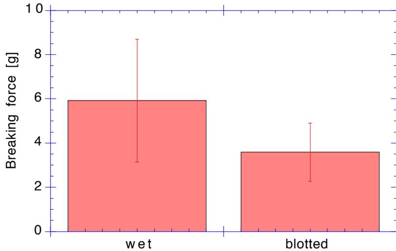
Figure 6: There was no significant difference between welding specimens that were dripping wet versus well blotted. Laser pulse energy was 2 J for this experiment 3. The slight differences in weld strength amongst tested specimens were more due to variation in ICG staining than due to wet vs blotted (see Figs. 7 and 8).
