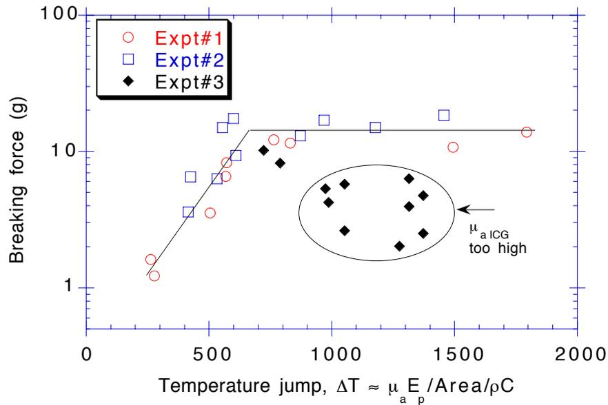
Figure 7: Weld strength increases with the peak temperature achieved by laser exposure. Breaking force of weld is plotted vs calculated temperature jump.
