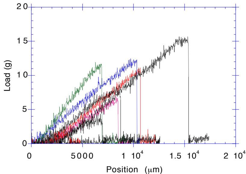
Figure 4: Stress-strain curves for elastin/carotid welds. Shows the curves for a set of welds created using different laser pulse energies. Weld made with lower energies broke at lower loads.
