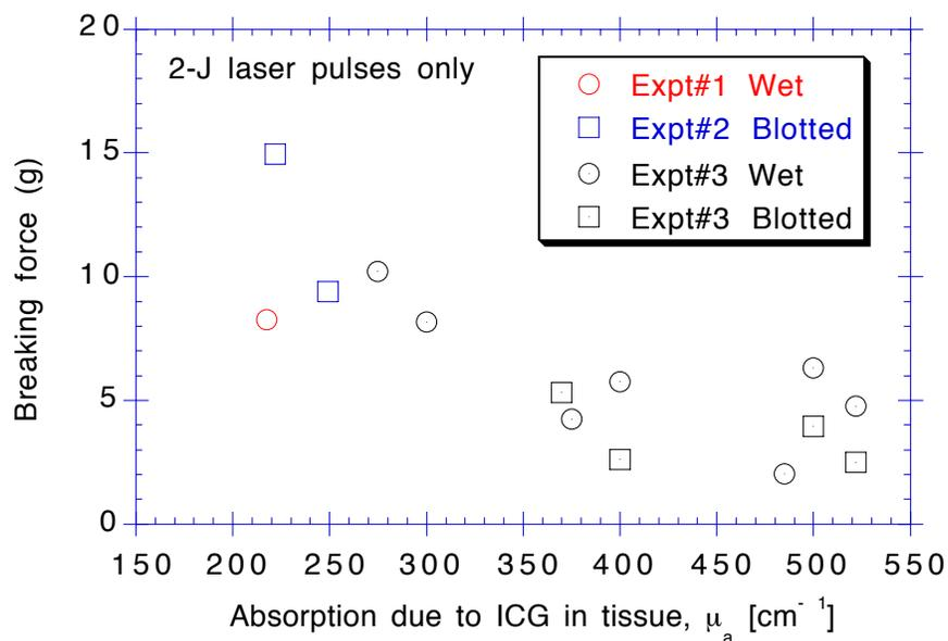
Figure 8: Weld strength decreases when the ICG staining was too high. The breaking force is plotted vs absorption coefficient of the ICG layer. Data shown are only those experiments involving 2-J laser pulses.
