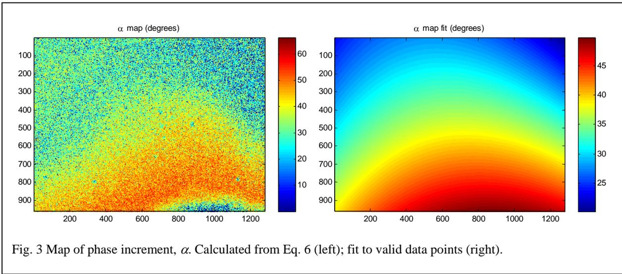
Fig. 3 Map of phase increment,  $\alpha$ . Calculated from Eq. 6 (left); fit to valid data points (right).
