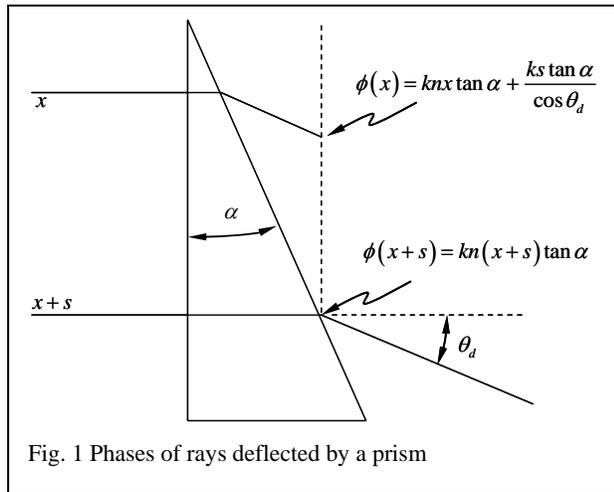
From Fig. 1 we see that the phase difference between the two rays separated a distance  $s$  (the image shear) is given by
