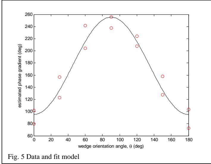
Note that the phase shown in Fig. 4 is actually the DIC phase difference for the wedge in this orientation. This phase distribution corresponds to an approximate  $\lambda/6$  variation in flatness, which is consistent with the tolerance on the wedge. Figure 5 displays the results of fitting the data to the model shown in Eq. 15.
