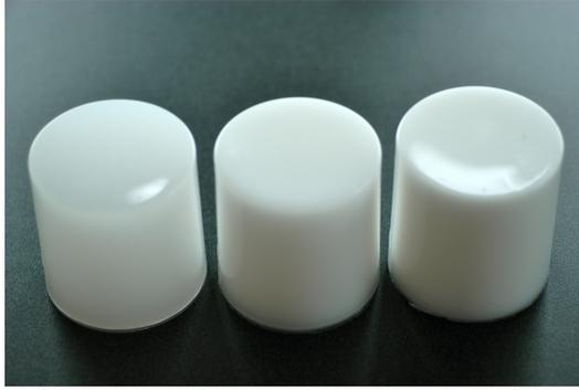
Figure 3: The three polyurethane phantoms with optical properties similar to tissue in the near infrared. Each phantom is 6 cm in diameter and 10 cm high. Left to right phantoms are identified as 1, 2, & 3.
