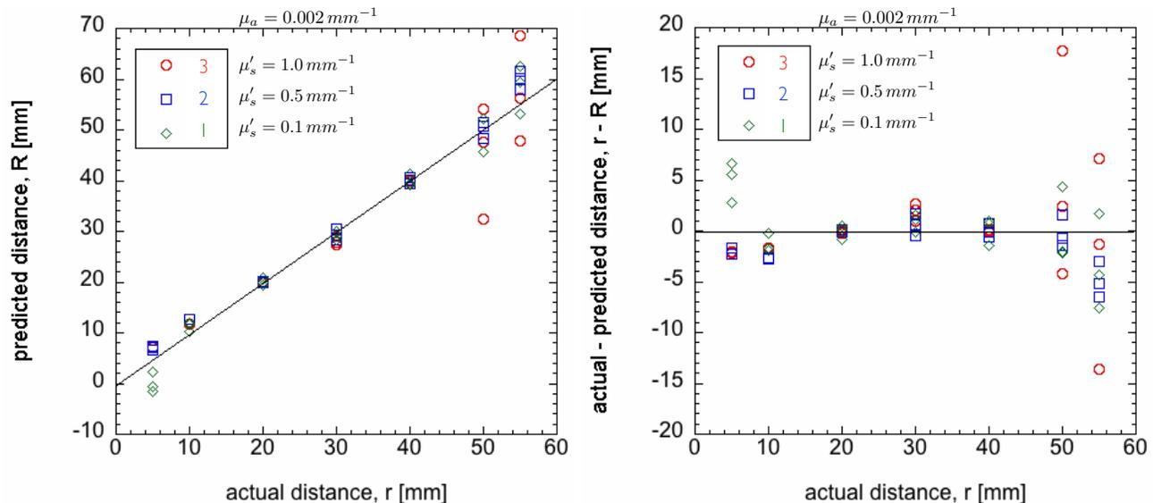
Figure 4: *Left*: The predicted distance plotted against the actual distance for each of the phantoms. The line is where the predicted distance equals the actual distance,  $R = r$ . *Right*: Residuals, the difference between the predicted distance and actual distance.
