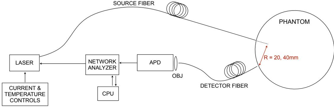
Figure 1: System used to measure the phase lag that develops between the source fiber (within the phantom) and the detector fiber (on the edge of the phantom) at  $R = 20$  &  $40$  mm. These two measurements were used to calibrate to the medium.
