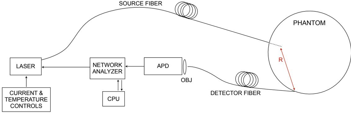
Figure 2: System used to measure the distance between the source fiber (within the phantom) and the detector fiber (on the edge of the phantom) at distances between 10–50 mm.
