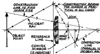
8 NEGATIVE (CONVEX) MIRROR ANY DISTANCE with OBJECT ANY DISTANCE
