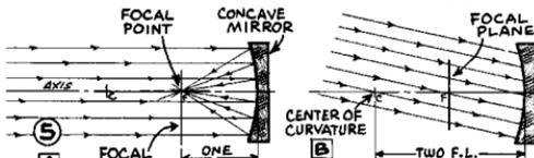
A BUNDLE OF PARALLEL LIGHT RAYS FROM A DISTANT AXIAL POINT WILL COME TO A FOCUS ON THE AXIS AT THE FOCAL POINT OF THE MIRROR
