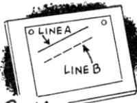
Problem: GIVEN THE SLANT LINE, A, HOW TO DRAW LINE B PARALLEL TO IT
