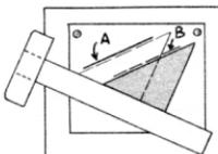
METHOD 2: SET A TRIANGLE TO LINE A AND THEN SLIDE IT ALONG HAND-HELD T-SQUARE TO DRAW LINE B
