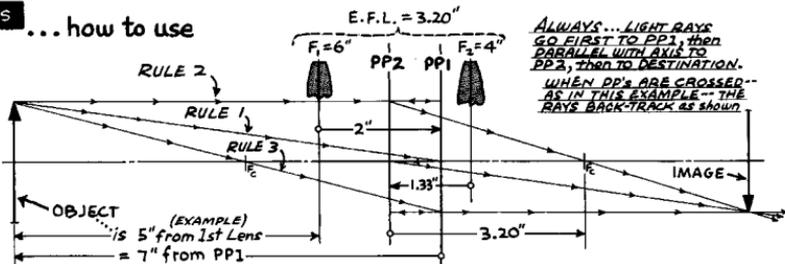
ALWAYS... LIGHT RAYS GO FIRST TO PP1, then PARALLEL WITH AXIS TO PP2, THEN TO DESTINATION. WHEN PP'S ARE CROSSED-- AS IN THIS EXAMPLE-- THE RAYS BACK-TRACK AS SHOWN.
