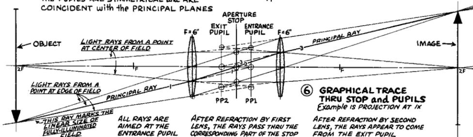
also locates the second principal plane as well as the rear focal point of the combined lenses.
