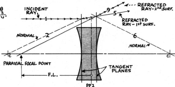
**VARIATIONS IN FOCAL LENGTH.** The various graph and math methods used to find  $f, l$ , may vary slightly since some of the methods are merely close approximations. For example, the  $f, l$ , of an equi-convex lens is the same as its radius of curvature-- $F=R$ . Neither glass thickness nor index are considered.
