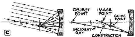
YOUR GUIDE IS THE RAY THAT PASSES THRU THE CENTER OF CURVATURE. THIS RAY IS NOT DEVIATED ... IT GOES TO THE MIRROR AND COMES RIGHT BACK AGAIN. THIS RAY COMES TO A FOCUS AT THE POINT WHERE IT CROSSES THE FOCAL PLANE
