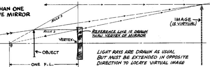
is also similar to the same construction for a lens. Notice that light rays in a mirror trace are bent at a straight reference line drawn through the vertex of the mirror; this is done to preserve the geometrical relationship which is the basis for this kind of graphical ray tracing. Actually you are not dealing with lenses or mirrors at all but only with similar triangles.
