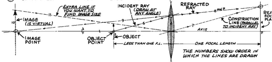
one focal length from a lens produces a virtual image on the same side of the lens as the object. A typical case is shown in Fig. 3. Ray tracing by the oblique method proceeds just the same as before, the only difference being that the refracted ray will be seen to be diverging and must be extended back toward the object in order to locate the axial image point.
