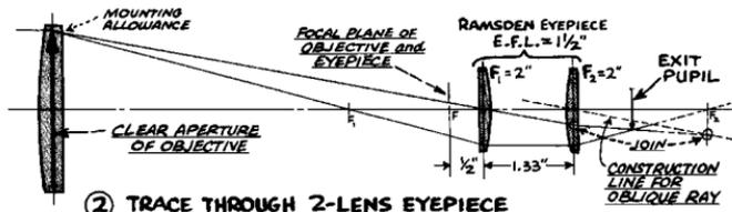
IN EVERY optical system there is one lens or diaphragm which limits the size of the bundle of light rays that can get through the lens system. This limiting aperture is called the aperture stop. Often it is the front lens of an instrument, which is the case for telescopes and microscopes. For a camera lens, the aperture stop is the iris diaphragm located between the lenses. When you use a magnifying glass, your eye is the smallest aperture in the optical system, and so becomes the aperture stop.
