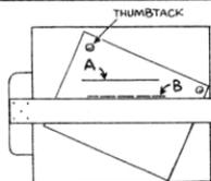
METHOD 1: RE-TACK DRAWING WITH LINE A PARALLEL TO T-SQUARE. YOU CAN THEN DRAW LINE B
